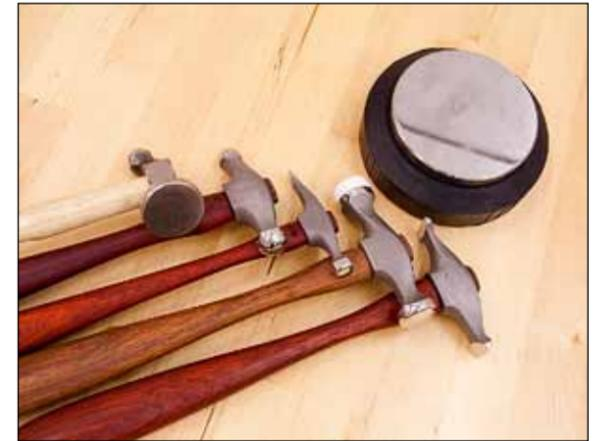
An assortment of hammers with a steel bench block in a rubber base.
