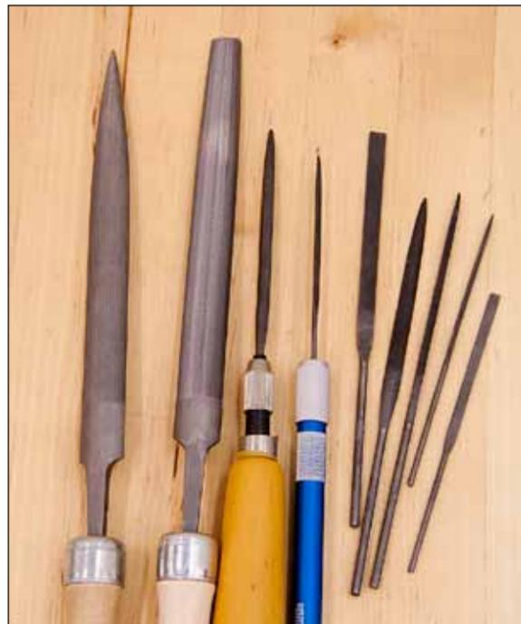
**Useful basic files (from left): #4 fine half-round file; #0 medium half-round file; half-round and round needle files in pin vise handles; assorted basic and mini needle files**
