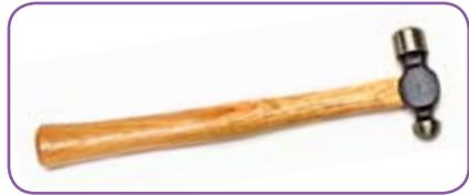
A **hammer** is used to harden and texture wire. Any hammer with a flat head will work, as long as the head is free of nicks that could mar your metal. The light ball-peen hammer shown here is one of the most commonly used hammers for jewelry making.
