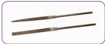
**Metal files** are used to refine and shape the edges of metal and wire surfaces.
