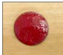
Underfired piece. The enamel has an orange-peel appearance.
